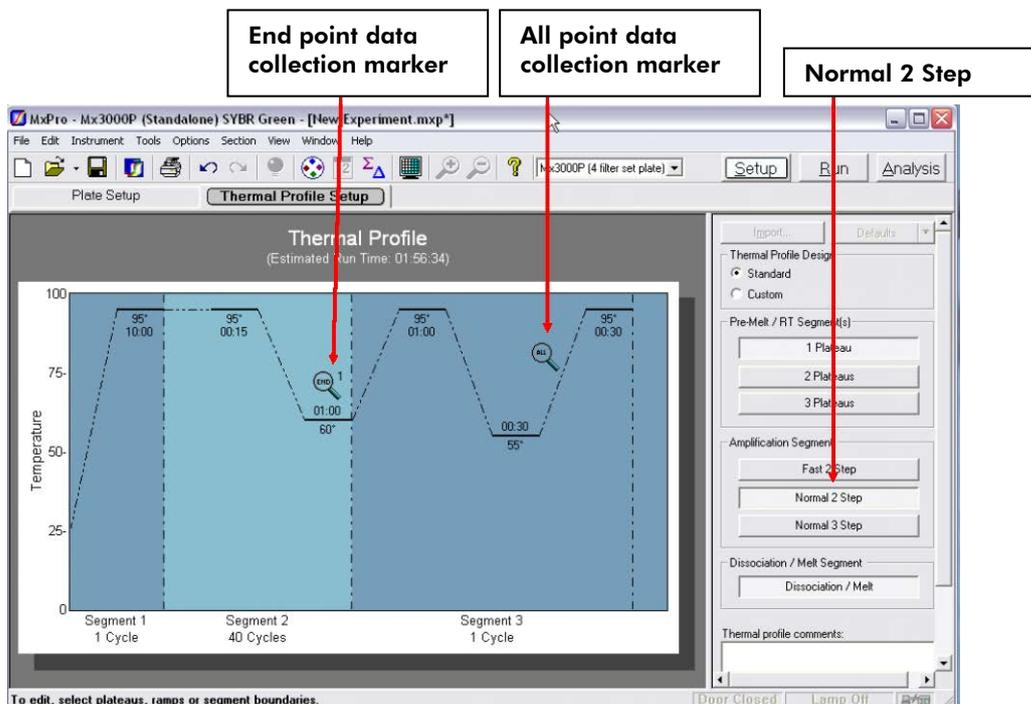
Figure 2. Thermal profile setup.
