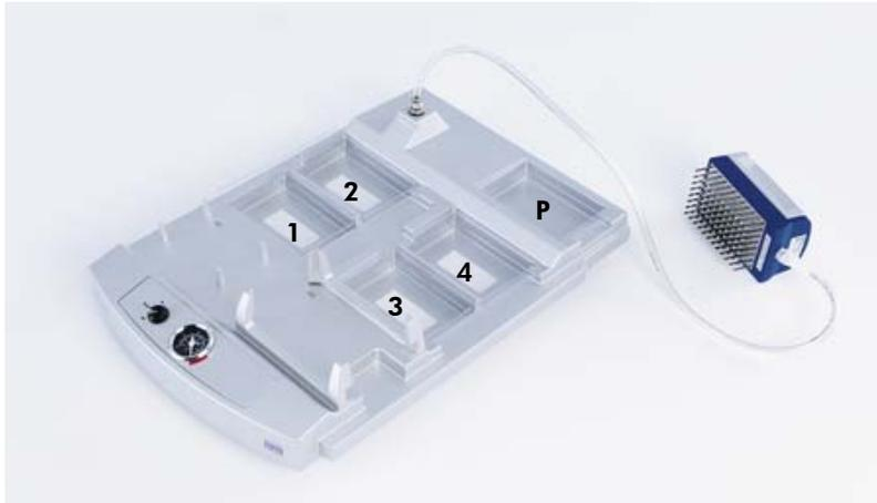
**Placement of PCR plate (or strips) and PyroMark Q96 Plate Low (PM Plate) on the PyroMark Q96 Vacuum Workstation.** The marked positions contain 70% ethanol (1), PyroMark Denaturation Solution (2), PyroMark Wash Buffer (3), and high-purity water (4).
