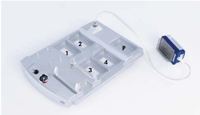
**Placement of PCR plate (or strips) and PyroMark Q96 HS Plate (PM Plate) on the PyroMark Q96 Vacuum Workstation.** The marked positions contain 70% ethanol (1), PyroMark Denaturation Solution (2), PyroMark Wash Buffer (3), and high-purity water (4).
