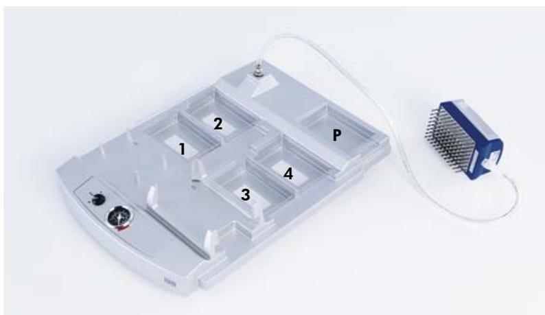
**Figure 3. PyroMark Q96 Vacuum Workstation.**
