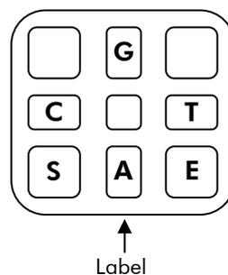
**Schematic diagram of the PyroMark Q96 Cartridge (viewed from above).** E: Enzyme Mixture; S: Substrate Mixture; G: dGTP; C: dCTP; T: dTTP; A: dATP $\alpha$ S.
