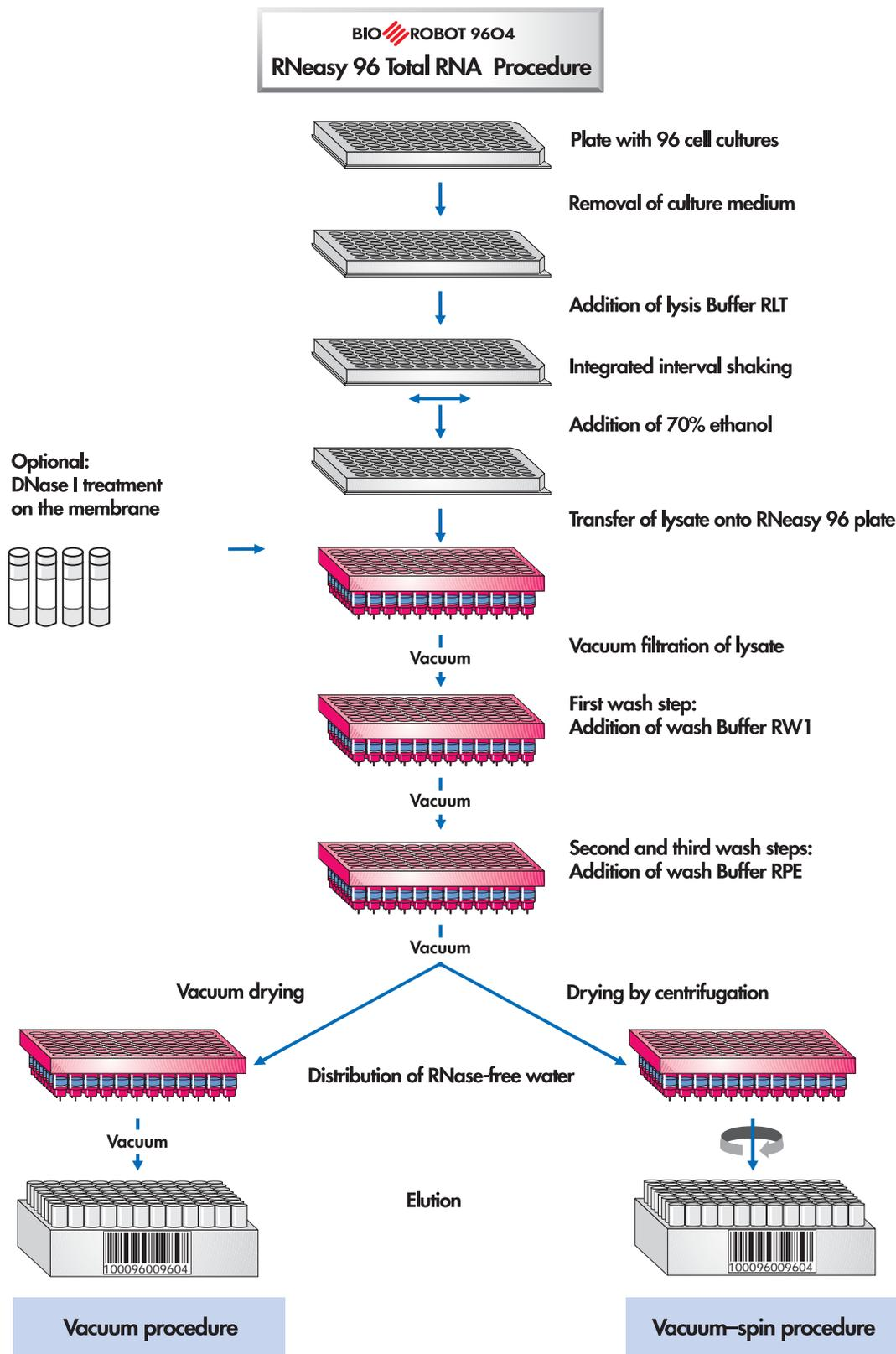
**Figure 1.** Total RNA isolation with the RNeasy 96 BioRobot 9604 Kit. Elution steps can be performed directly on the BioRobot 9604 or in a specially designed centrifuge system (see page 9).
