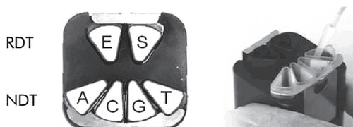
**Figure 1. Illustration of the PyroMark Q96 HS Dispensing Tip Holder seen from above.** The annotations correspond to the label on the reagent vials. **E:** Enzyme Mixture; **S:** Substrate Mixture; **A, C, G, T:** nucleotides.
