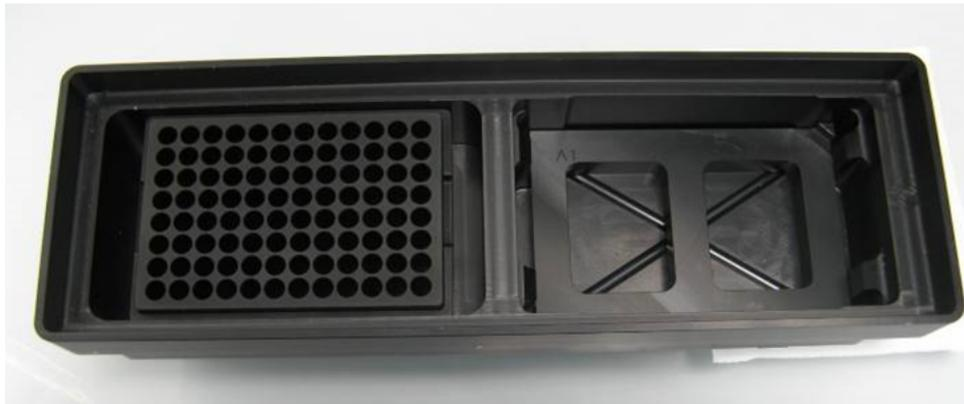
4. Place the transfer carriage (4) onto the left (waste) chamber of the vacuum chamber (1). Ensure that the transfer carriage is positioned to the left inside the left (waste) chamber of the vacuum chamber.
