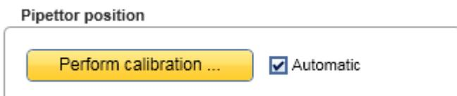
3. Click the **Perform calibration...** button. The pipettor head ejects the tips, picks up a new column of tips and moves to the calibration position.
