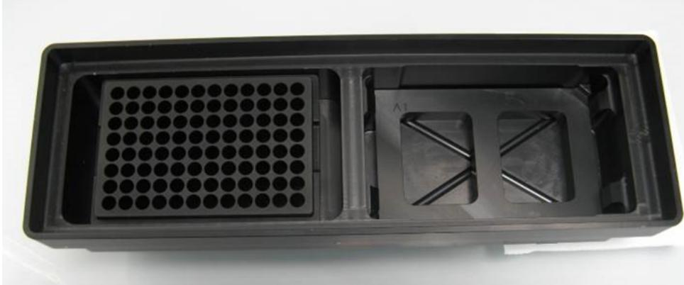
**Note:** For worktable position A1, the calibration needs to be performed into the channeling adapter only (i.e., without a filter plate) to increase calibration precision.
