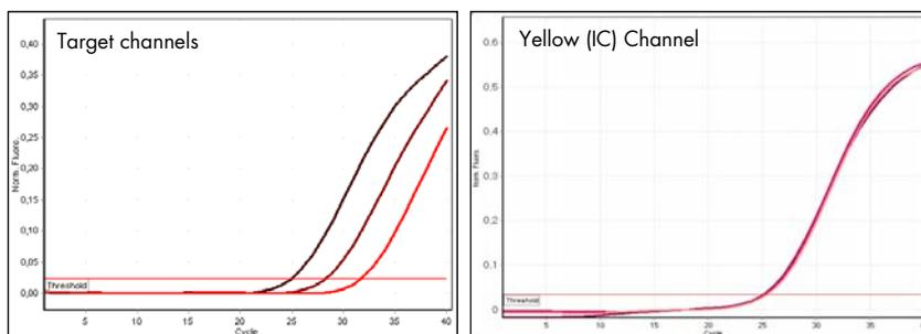
**Figure 2. The sample is positive for tested pathogen.** The 3 sample curves in the target channel (left) are above a preset threshold indicating the presence of pathogen DNA. The corresponding curves of the internal control in the Yellow Channel (right) are above the threshold and have a  $C_T$  value of 24–28, indicating that the PCR was successful and not inhibited.
