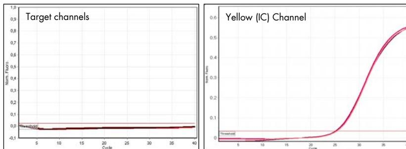
**Figure 1. The sample is negative for tested pathogen.** The 3 sample curves in the target channels (left) are at the baseline and below a preset threshold. The corresponding curves of the internal control in the Yellow Channel (right) are above the threshold and have a  $C_T$  value of 24–28, indicating that the PCR was successful and not inhibited.
