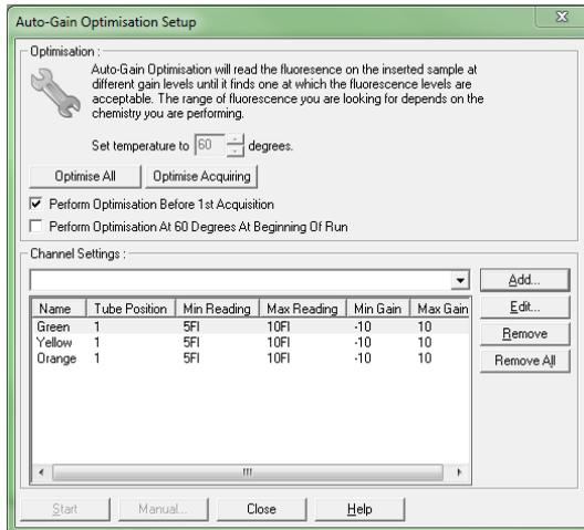
**Perform Gain Optimization for the 3 channels before 1st acquisition.**
