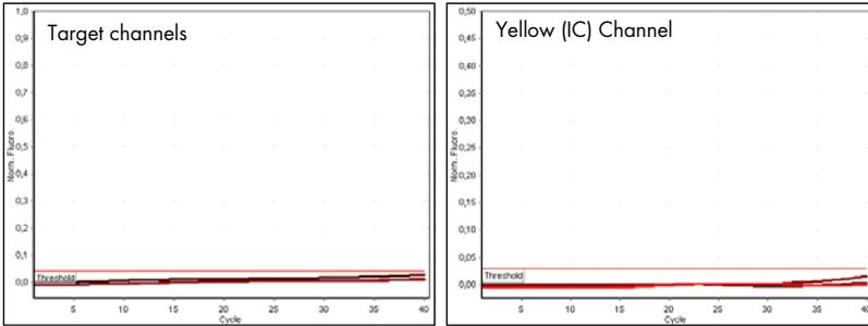
**Figure 3. The PCR is inhibited.** No amplification of the 3 samples in the target channel (left) or the internal control in the Yellow Channel (right). All curves lie along the baseline and do not exceed a preset threshold.
