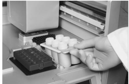
**Figure 17: Loading the reagent bottle rack. [A]** Schematic of positions and contents of bottles in the reagent bottle rack. **[B]** Loading the rack onto the QIAcube Connect MDx.
