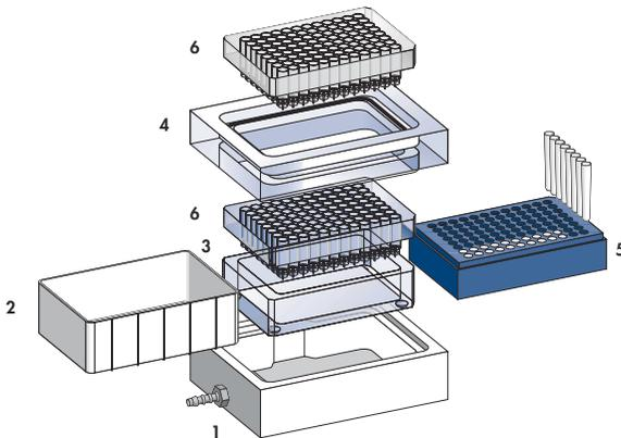
**Figure 3** Exploded diagram of QIAvac 96 and components
