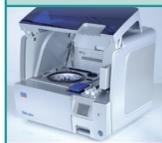
**The QIAcube.** The QIAcube instrument is a robotic system for biological sample preparation that includes a liquid handling unit, a robotic arm with grabber, a centrifuge, and a thermoshaker unit.
