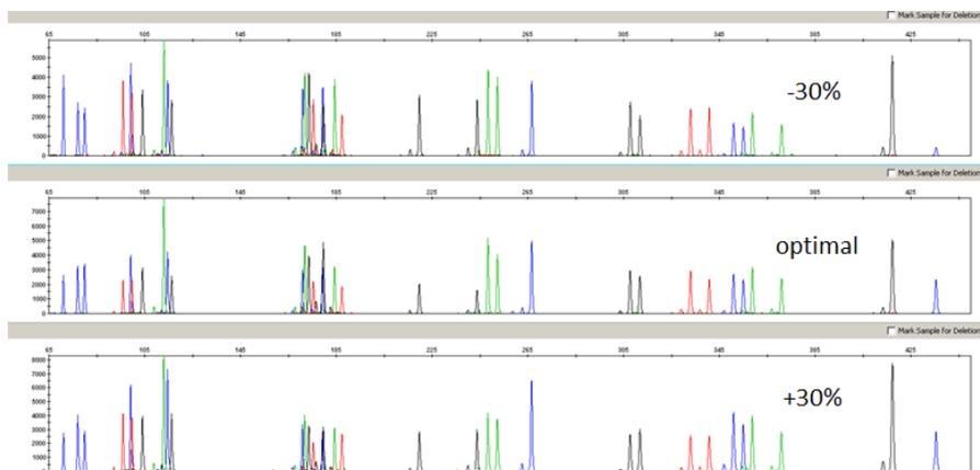
**Figure 1. Influence of MgCl<sub>2</sub> concentration.** Fast Reaction Buffer 2.0 (FRM 2.0) was supplemented with different concentrations of MgCl<sub>2</sub> matching the specification of production, or 30% higher or lower. Representative electropherograms of sample quadruplicates are shown.
