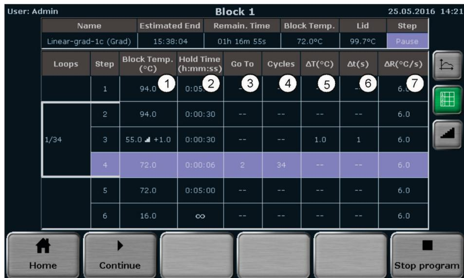
Figure 25. QIAmplifier 96 spreadsheet program view.
