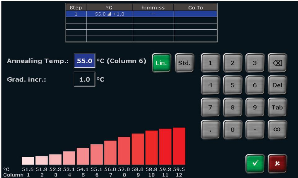
Figure 23. QIAmplifier 96 Linear Gradient Tool screen.
