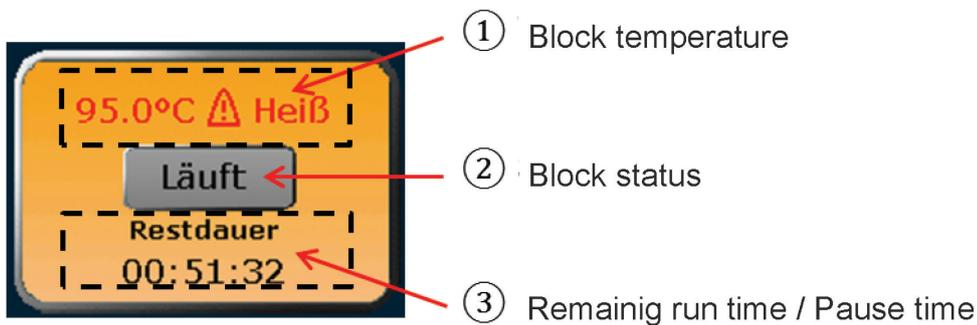
Figure 12. QIAmplifier 96 block status/quick start button.
