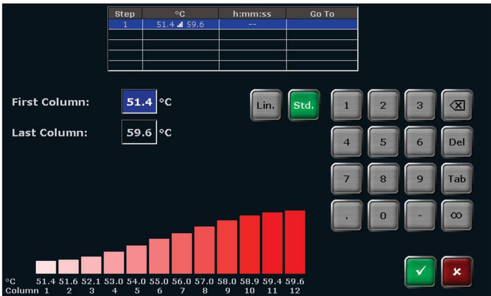
Figure 24. QIAmplifier 96 standard gradient programming screen.
