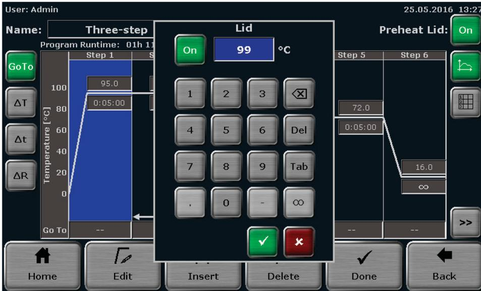
Figure 20. QIAmplifier 96 heated lid temperature setting screen.
