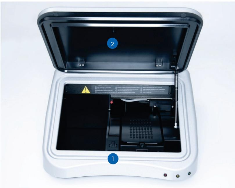
Figure 5. View of the optical sensor when the access door is opened. (1): Optical sensor (2): Flag
