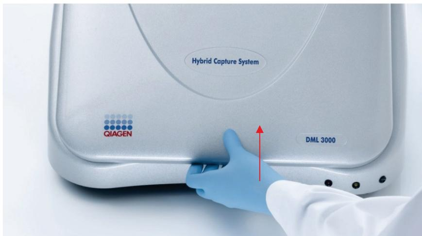
Figure 3. Opening the access door of the DML 3000
