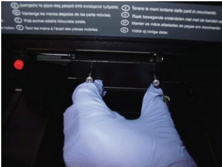
Figure 40. Removing the optical mask.
