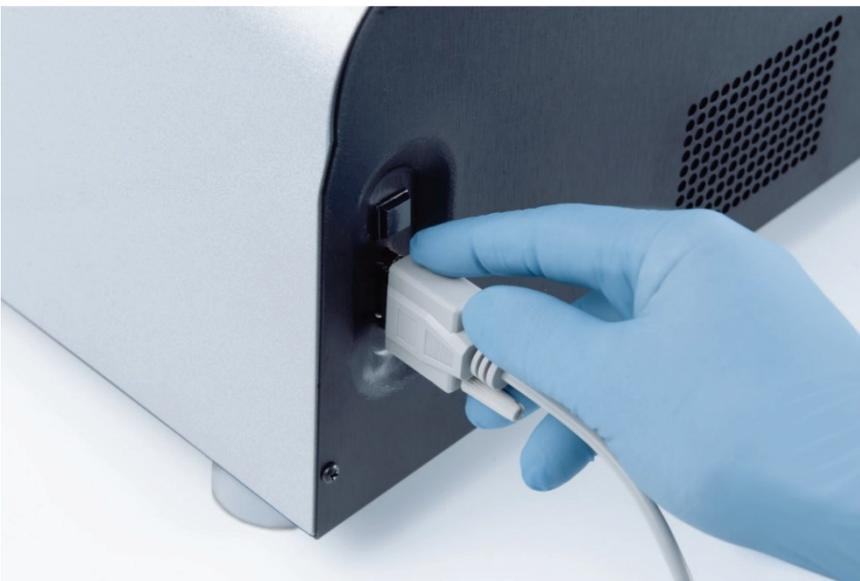
Figure 22. Close-up view of the RS-232 port
