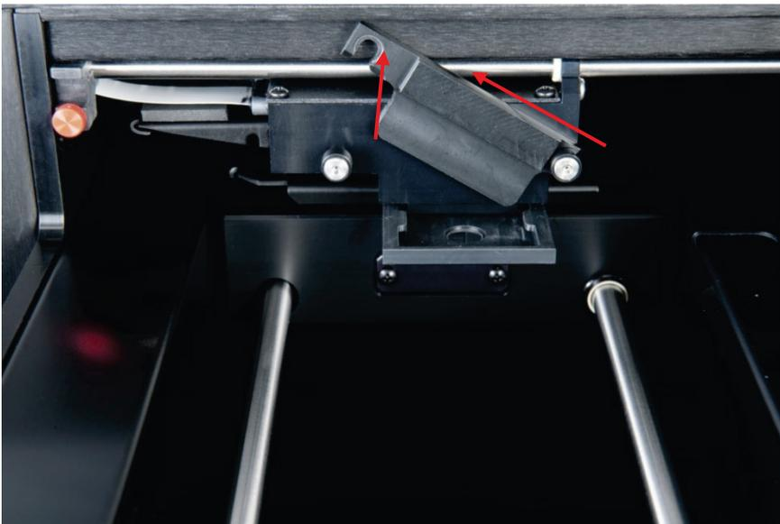
Figure 39. Removing the optical mask retainer
