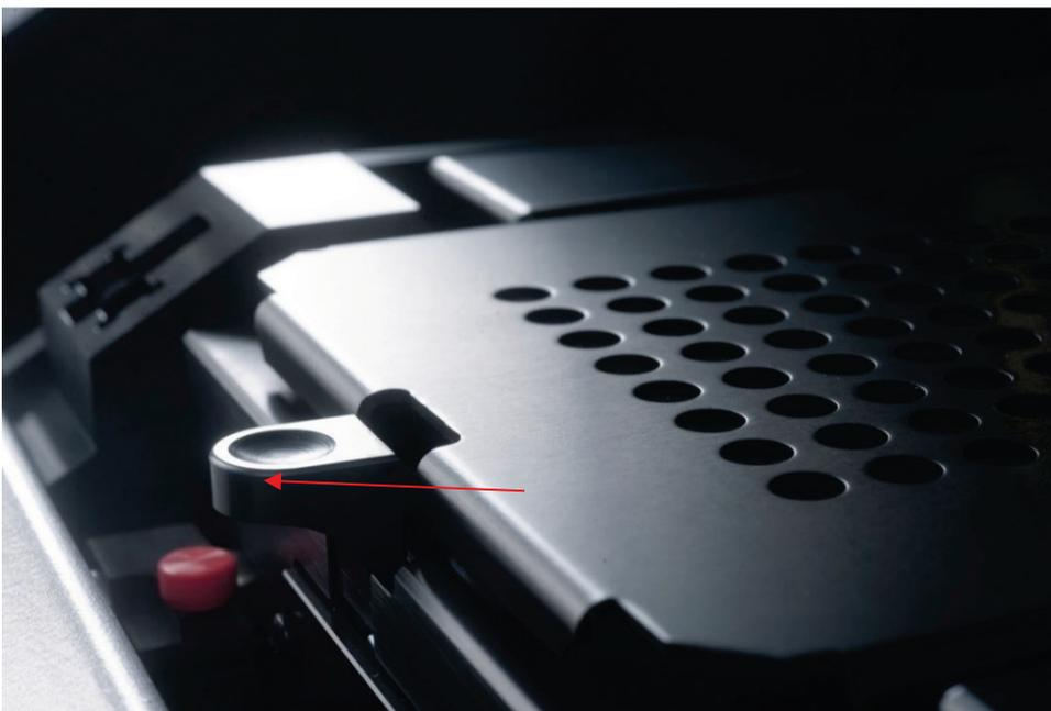
Figure 9. View of the plate mask release latch
