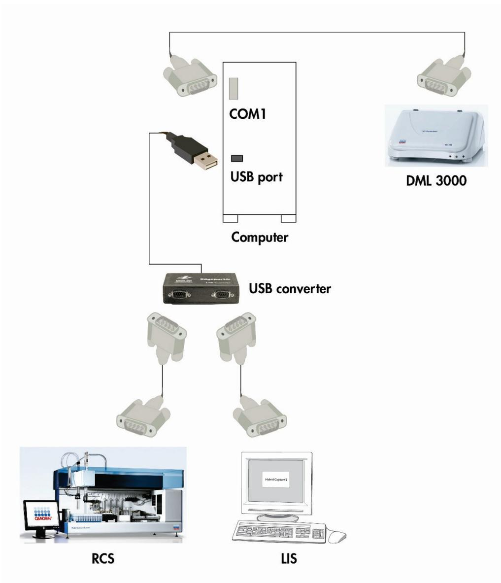
Figure 26. Diagram of connecting a DML 3000 with a RCS and a LIS.
