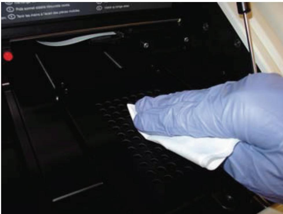
Figure 33. Wiping the top of the plate mask
