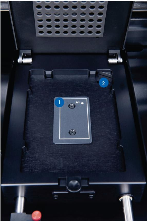
Figure 10. View of the microplate locator. (1): Microplate locator (2): A1 orienting corner
