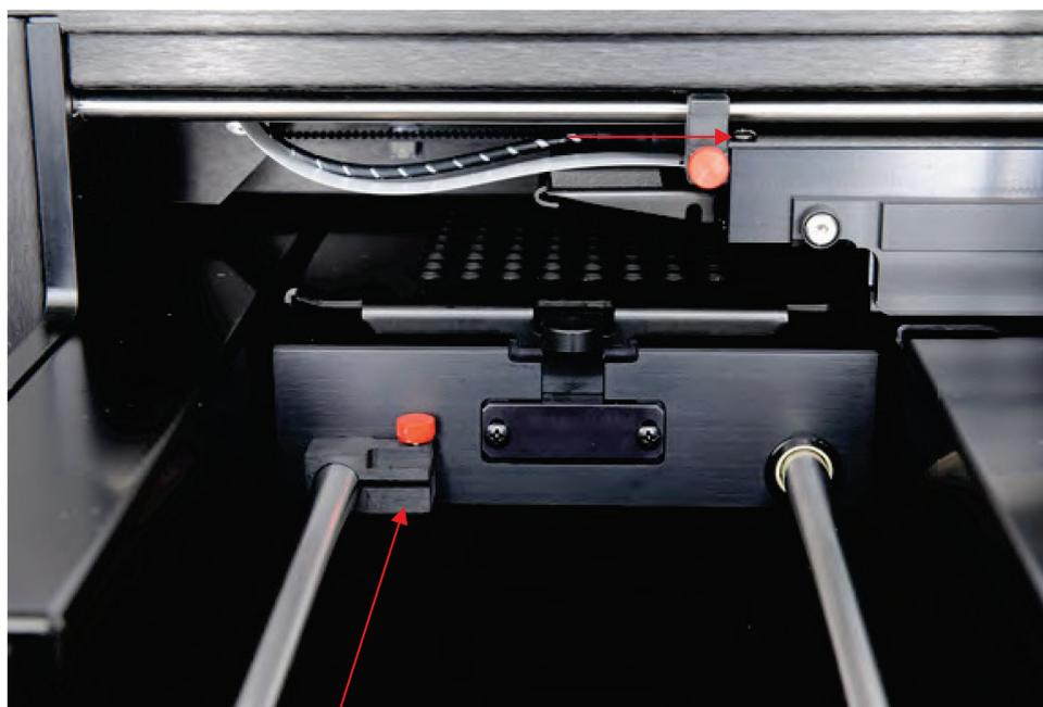
Figure 12. View of the transport locks in the secured position and ready for transport
