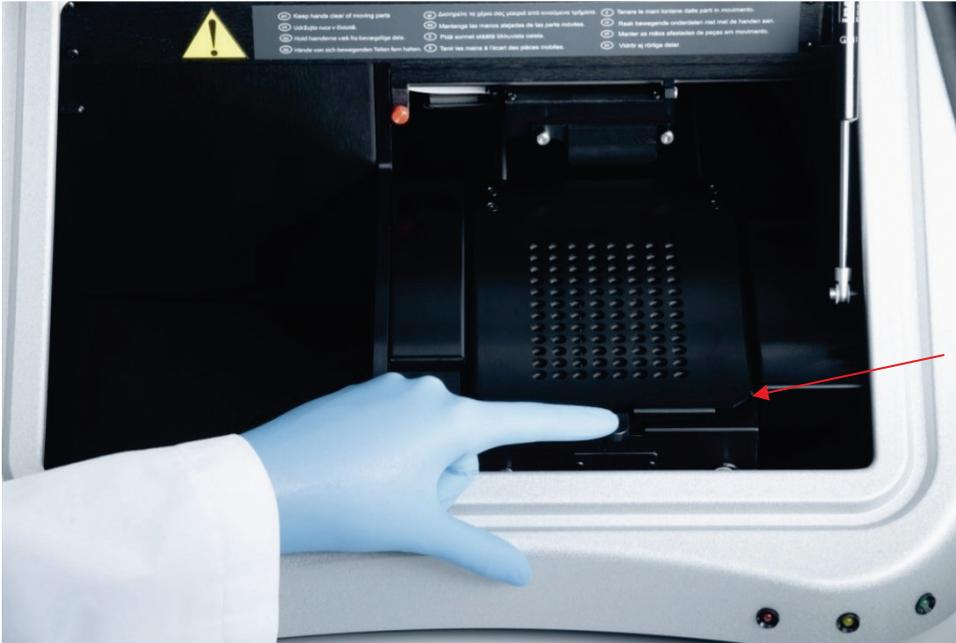
Figure 8. View of the plate mask when the access door is opened
