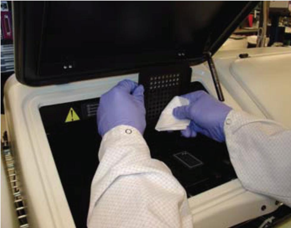
Figure 34. Wiping the interior of the plate mask
