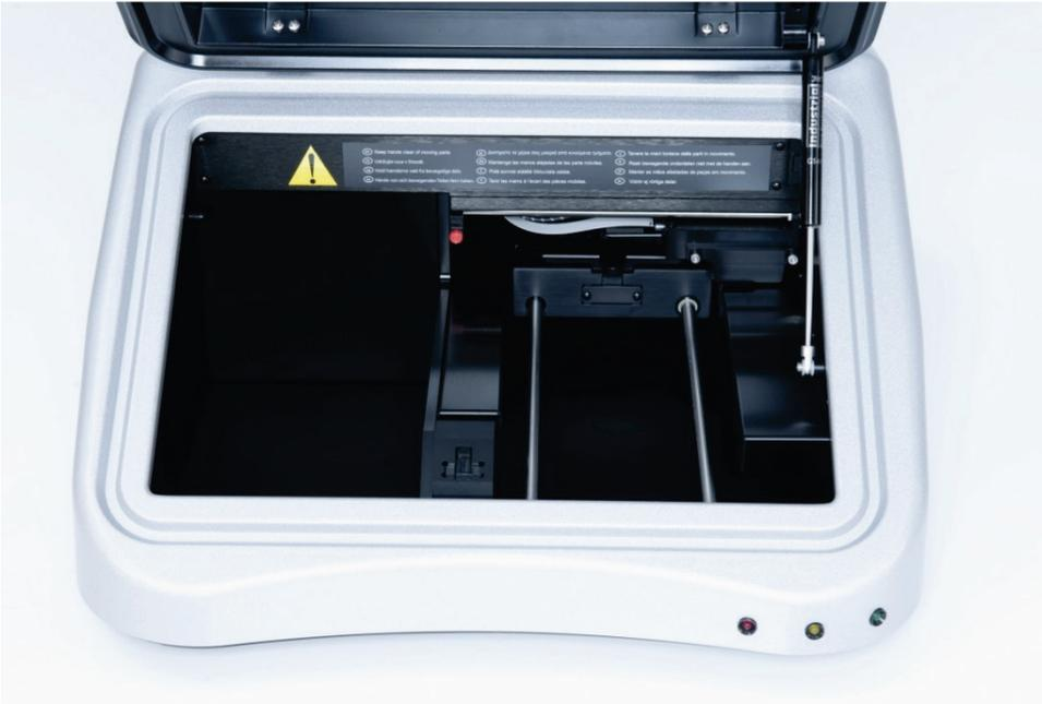
Figure 30. View of the plate carrier pushed to the back of the DML 3000
