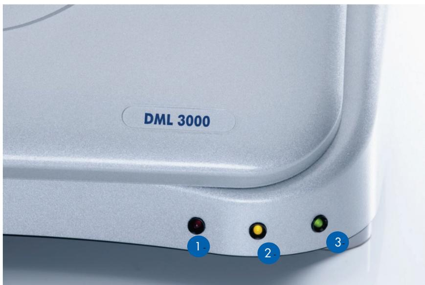
Figure 2. View of the LED status lights. (1): Red Led status light (2): Yellow Led status light (3): Green Led status light
