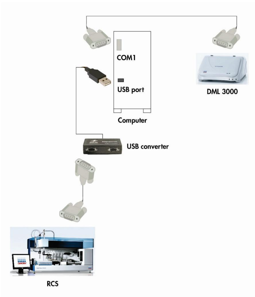
Figure 24. Diagram of connecting a DML 3000 with an RCS.
