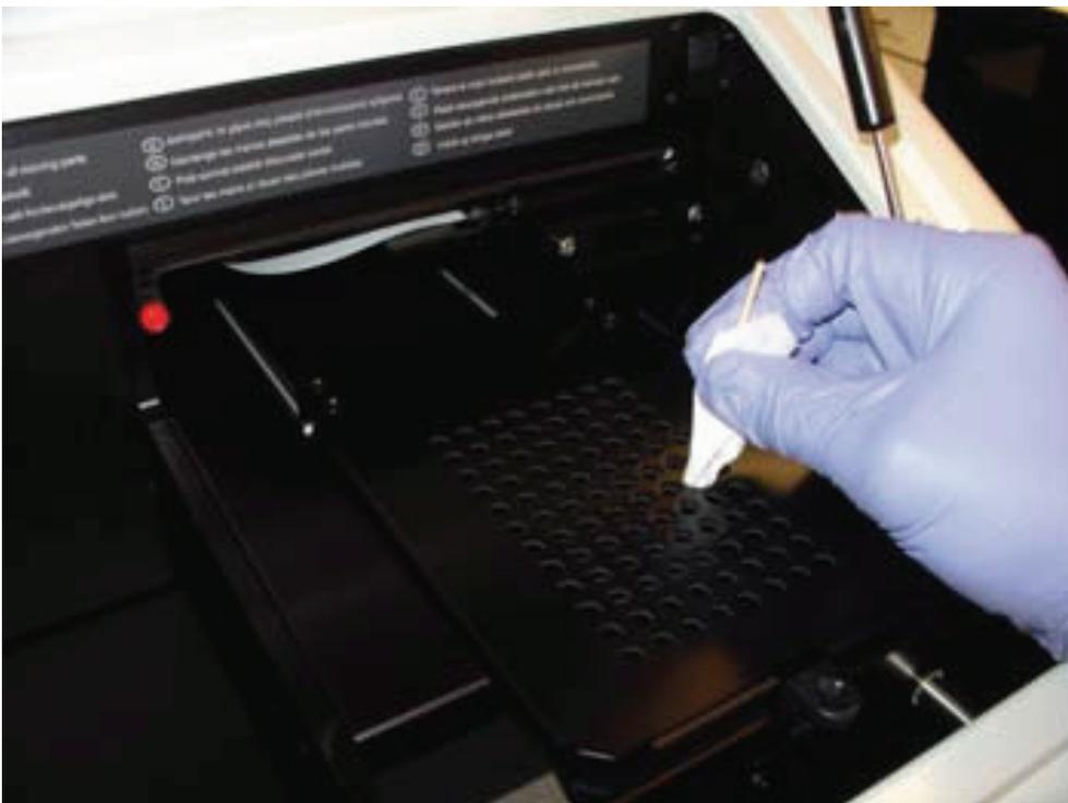
Figure 35. Cleaning the plate mask openings
