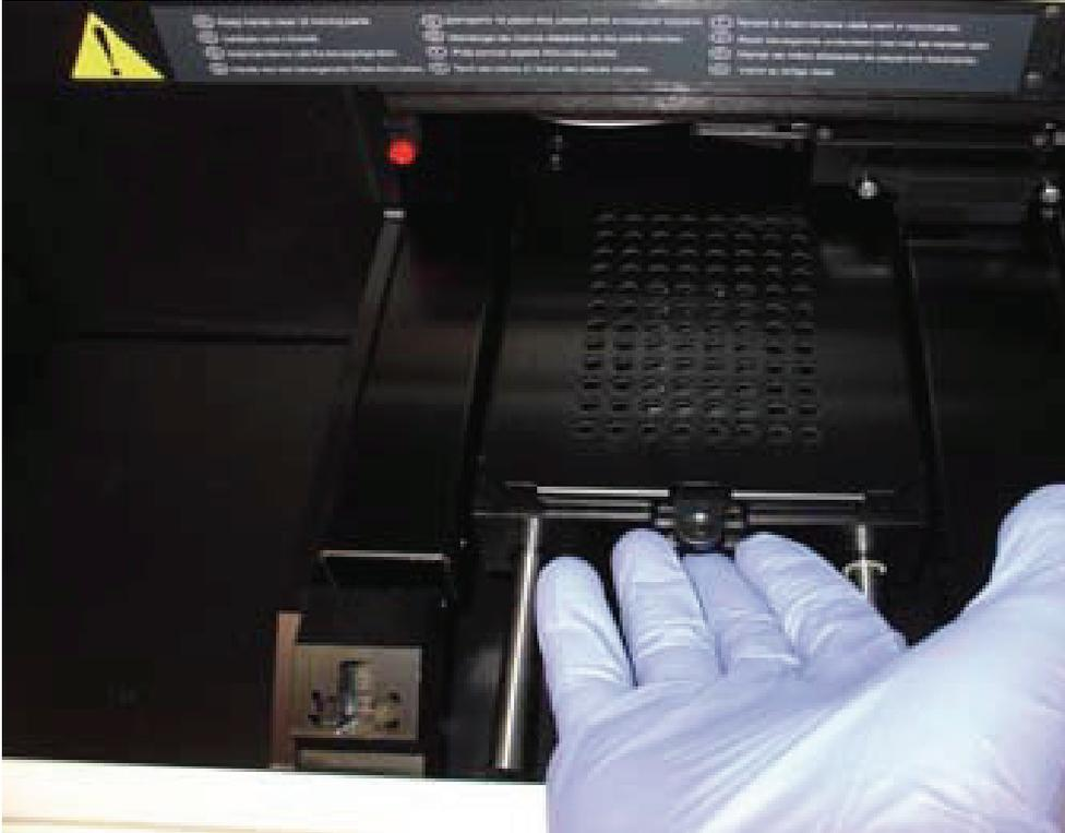
Figure 36. Pushing the plate carrier
