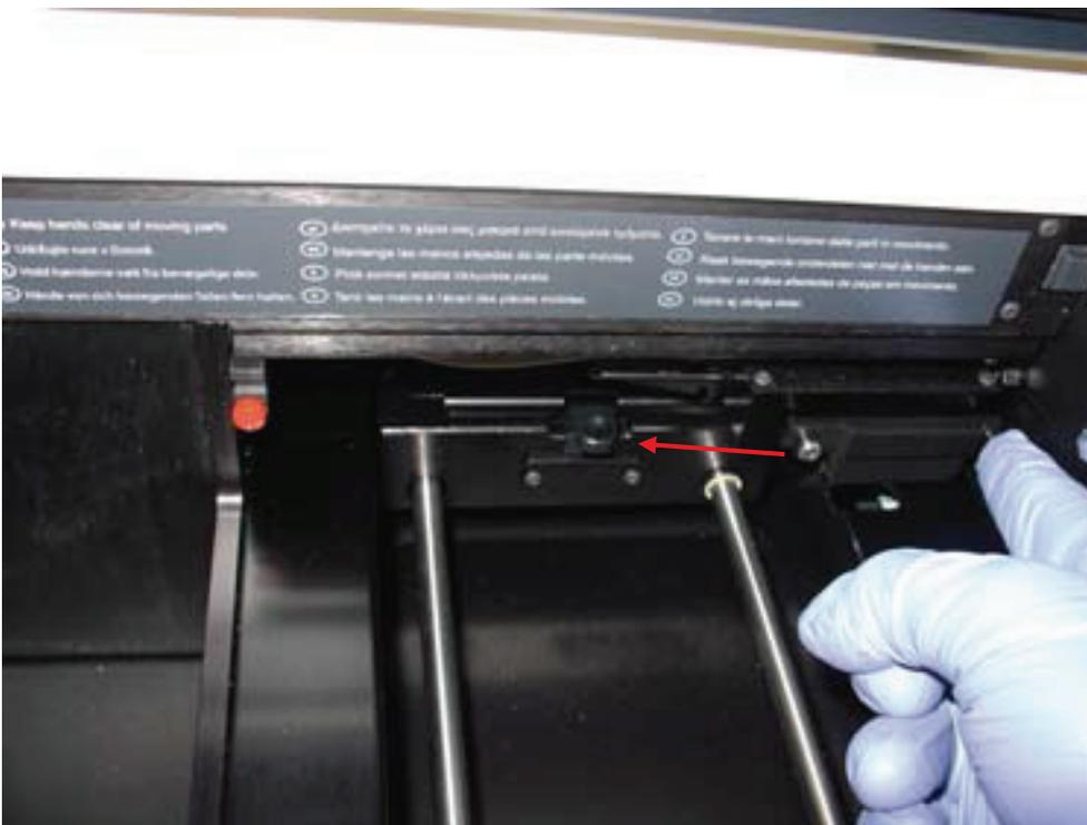
Figure 37. The optical head in the home position
