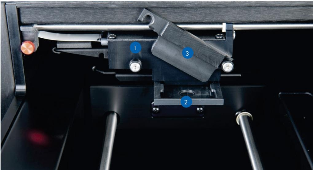
Figure 7. Close-up view of the optical head. (1): Optical head (2): Optical mask (3): Optical mask retainer
