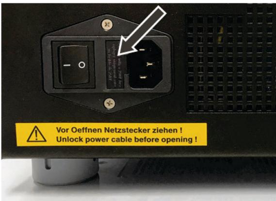
Figure 10. Fuse holder on the rear of the device.
