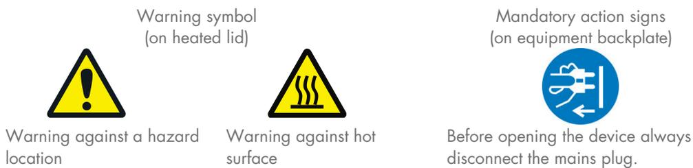
The following notice sign is attached to the rear of the QIAquant 96:
