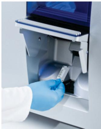
23. After loading the priming flow cell, manually close the flow cell door.
