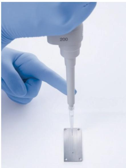
Figure 2. Correct dispensing technique for transferring beads to the flow cell port.
