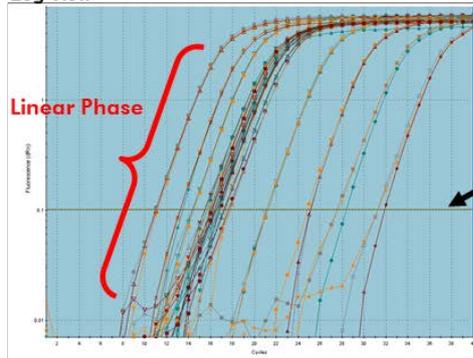
Set the threshold above the background signal but within the lower third of the linear phase of the amplification plot.
