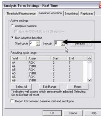
Set the baseline from cycle number 2 through two cycle values before the earliest visible amplification.
