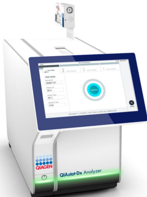
Figura 15. Inserindo o QIAstat-Dx Respiratory SARS-CoV-2 Panel Cartridge no QIAstat-Dx Analyzer 1.0.
