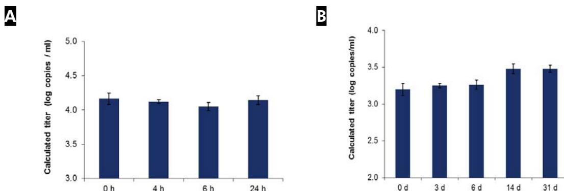
**Figure 4. Stability of CMV in eluates.** CMV standard material spiked in urine was purified on the QIAAsymphony SP using the Complex 200 protocol. Eluates were incubated **A** for 24 hours at 37°C and **B** for 31 days at 5°C. An in-house real-time PCR assay for CMV was used for detection at regular timepoints. Eluates were analyzed in replicates of 8.
