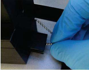
2. Grasp the chain connected to the tip ejector chute.
