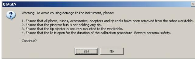
6. Open the instrument lid and ensure that the worktable has been cleared.
