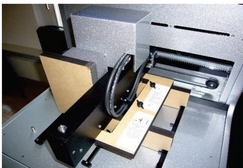
1. Unscrew the two screws (1 and 2) and remove the horizontal bar.
