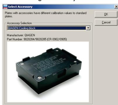
3. Select the required accessory from the drop-down menu. An image of the accessory will appear. Alternatively, to remove an accessory, select **No accessory** from the drop-down menu.
