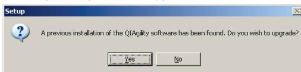
10. To uninstall a previous software version, click on the **Yes** button. The calibration settings and run files will be retained. To maintain the previous version of the software, click on the **No** button and browse for a different installation directory. Click on the **Next** button to continue.
