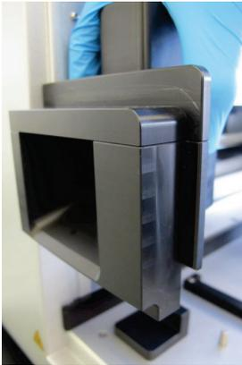
4. Remove the tip ejector/tip ejector chute.
