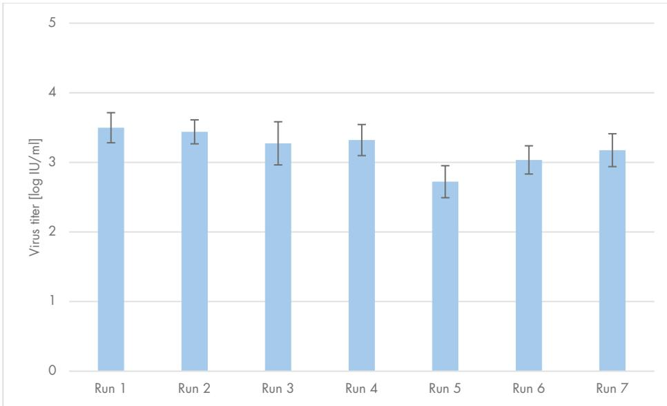
**Figure 5. Intra-run precision using the EZ1 DSP Virus system.** Stool samples were collected, pooled and prepared with the respective virus titer before use. NA was purified from 200 µl aliquots in 7 runs of 9/10 replicates each on the EZ1 Advanced XL. Mean virus titer and standard deviation are shown for each run.
