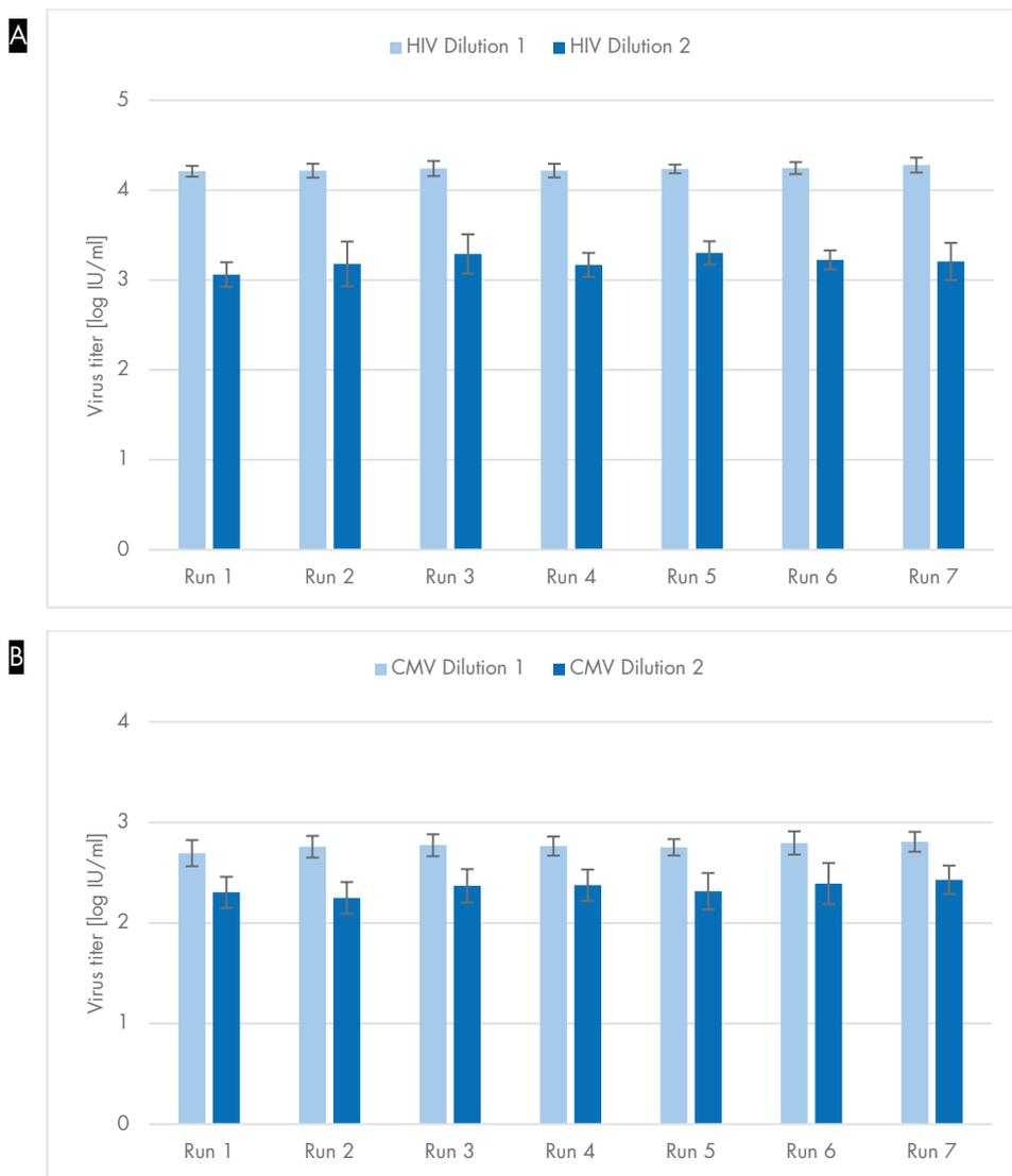
**Figure 4. Intra-run precision using the EZ1 DSP Virus system.** Plasma was collected, pooled, and prepared with the respective virus titer before use (A: HIV; B: CMV). NA was purified from 400 µl aliquots in 7 runs of 14 replicates each on the EZ1 Advanced XL using the EZ1 DSP Virus system. Mean virus titer and standard deviation are shown for each run.
