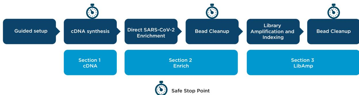
**Figure 1.** QIAseq<sup>®</sup> DIRECT enhanced SARS-CoV-2 automated workflow for the Biomek i7 Hybrid Automated Workstation System.
