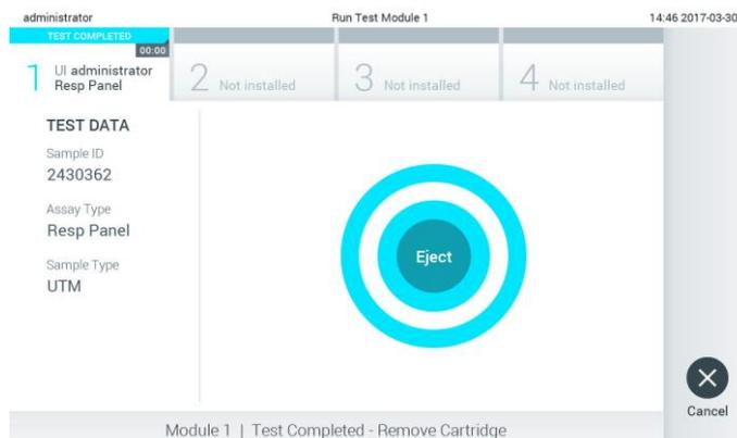
**Prompt to eject the used cartridge after running a test.**
