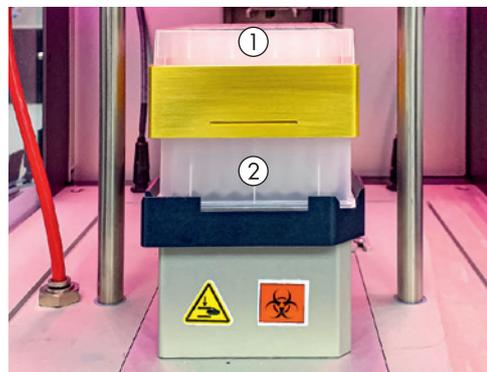
**Figure 9.** Plasmid *Plus* 96 Plate and elution plates were placed on the Resolvex A200 for dispensing of Buffer EB. A slow pressure gradient was applied to elute the samples. To maximize recovery, the elution step was performed twice. 1: Plasmid *Plus* 96 Plate. 2: Elution plate.
