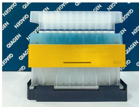
Figure 3. TurboFilter 96 Plate placed on top of a QIAprep 96 Plate and deep-well plate with adapters.
