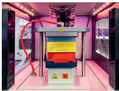
Figure 4. QIAprep 96 Plate placed for DNA binding and washing steps, using adapters to fit under the pressure head.
