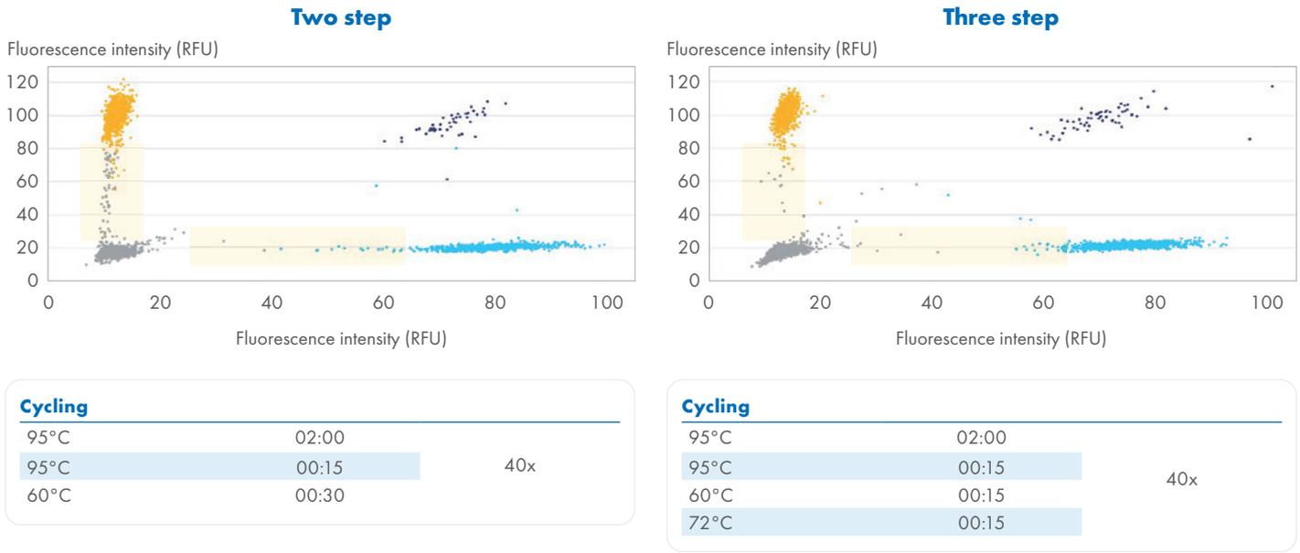
**Figure 8. Transition from two- to three-step thermal cycling can improve separation.** 100 copies/ $\mu$ l wild-type gDNA samples were tested with CDH1 (FAM)/TERT (HEX) in a duplex reaction. QIAcuity Probe PCR Master Mix was used. The cycling parameters are as indicated in the table, and the standard QIAcuity imaging setup was used. This adaptation improves the cluster separation.
