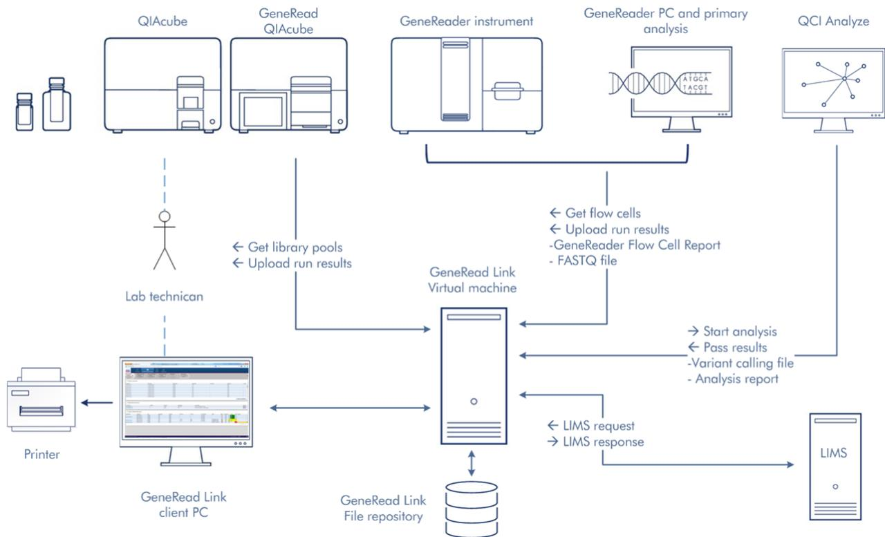
The figure above shows an example of the integration of GeneRead Link software into the GeneReader NGS System and with a LIMS. It also shows the exchange of data between the software components.
