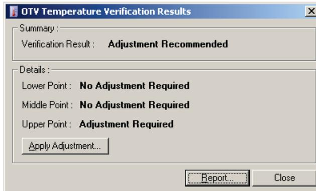
6. When the run is finished, the software indicates whether the Rotor-Gene Q MDx is within specification.
