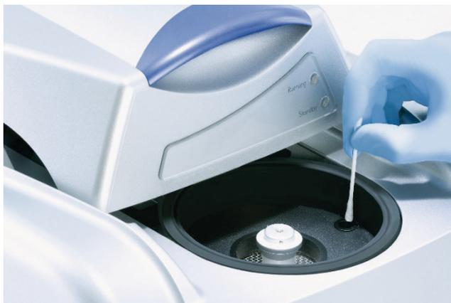
To avoid dust build up, keep the lid of the Rotor-Gene Q MDx closed when the instrument is not in use.
