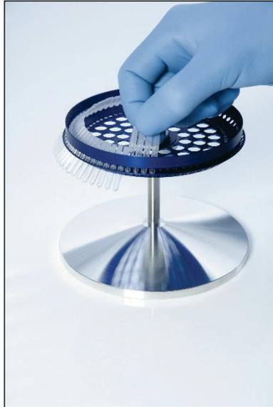
**Important:** To achieve maximum temperature uniformity, each position in the rotor must contain a tube. Filling all positions in the rotor ensures even airflow to every tube. Keep a set of empty capped tubes available that can be used to fill any unused positions.
