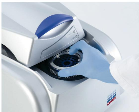
6. Close the lid and set up the run profile using the Rotor-Gene Q software.
