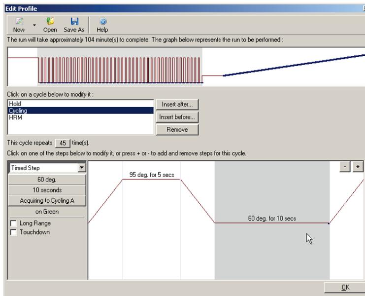
7. Ensure fluorescence data will be acquired. Acquire data to the green channel at the end of the anneal step.
