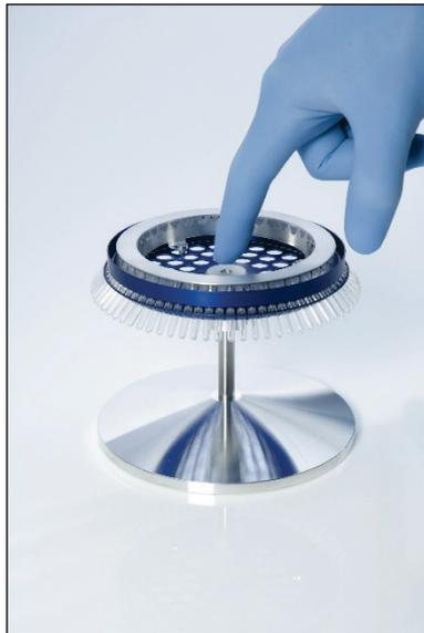
5. Insert the assembly into the Rotor-Gene Q MDx chamber by clicking into place using the locating pin on the rotor hub. To remove, simply push down on the rotor hub to release and pull out.
