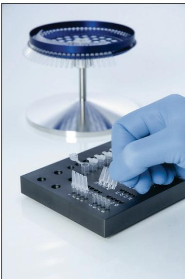
3. Insert the Strip Tubes into the 72-Well Rotor, ensuring that each tube sits correctly in place in the correct orientation.
