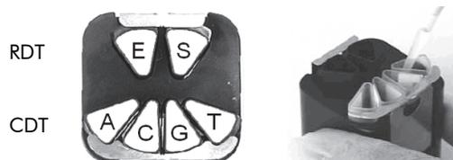
**Figure 1: Illustration of the PyroMark Q96 Capillary Tip Holder seen from above.** The annotations correspond to the label on the reagent vials. **E:** Enzyme Mixture; **S:** Substrate Mixture; **A, C, G, T:** nucleotides.
