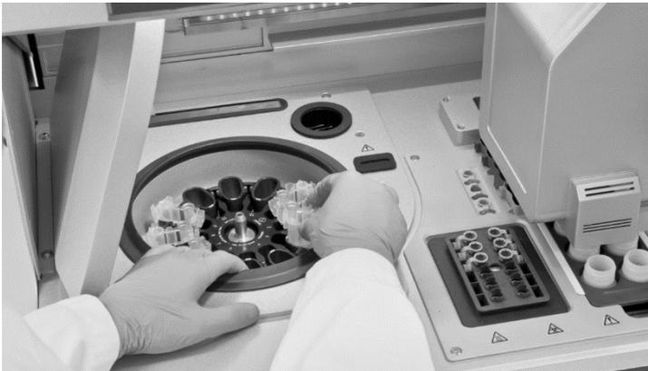
**Figure 21. Loading the centrifuge on the QIAcube instruments.** Load the assembled rotor adapters into the centrifuge buckets (QIAcube Connect MDx shown as example).
