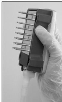
Figure 4. Illustration of the vacuum tool raised to beyond 90° vertical.
