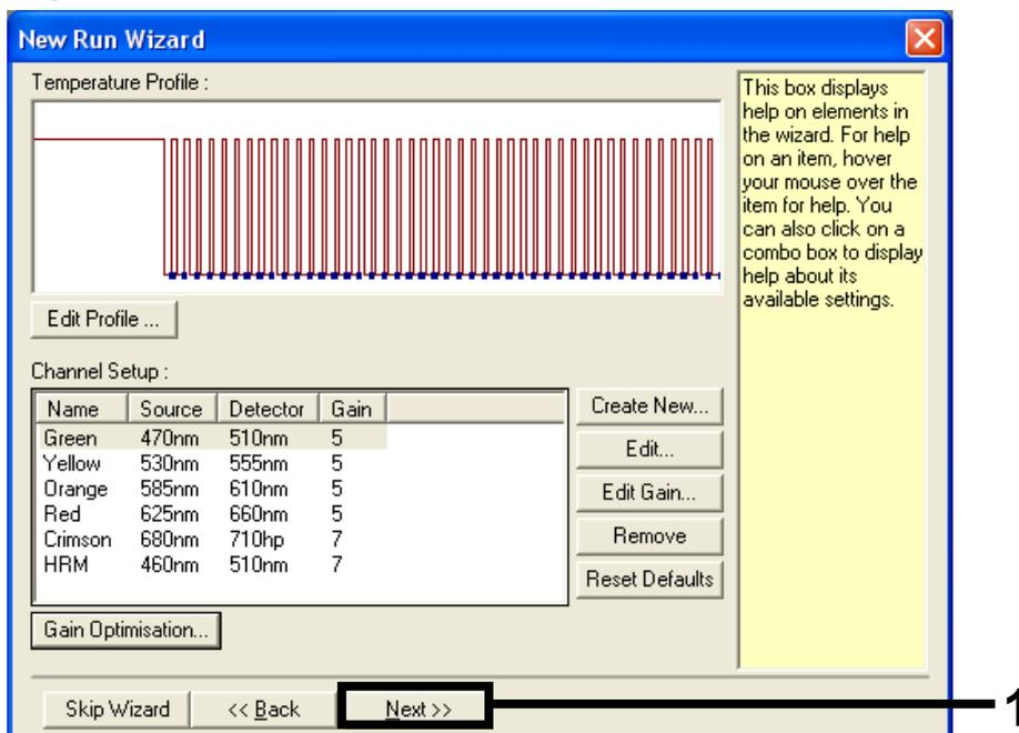
Figure 35. The "New Run Wizard" dialog box and temperature editing screen (1 = "Next" button).
