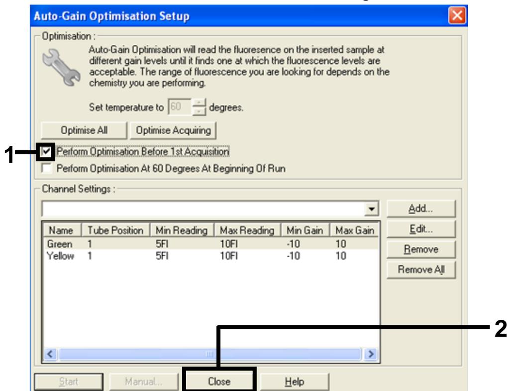
Figure 31. Selection of Green and Yellow channels (1 = "Perform Optimisation Before 1st Acquisition" tick box; 2 = "Close" button).
