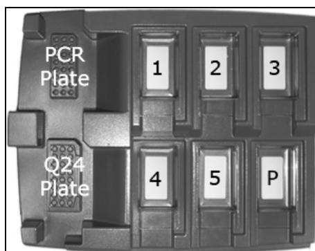
**Figure 3. Placement of PCR plate and PyroMark Q24 Plate on the PyroMark Q24 MDx Vacuum Workstation.** The marked positions contain 70% ethanol (1), PyroMark Denaturation Solution (2), PyroMark Wash Buffer (3), and high-purity water (4, 5). P: Parking position.
