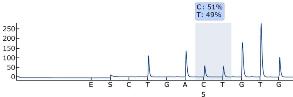
**Figure 5. Example of AQ assay result from a 50% mix (tube "C0.1").**
