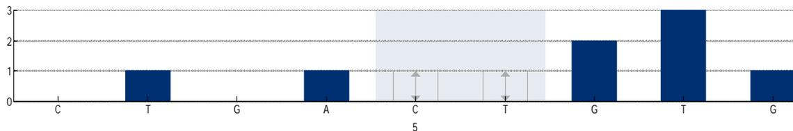
**Figure 2. Histogram for AQ mode.** The first and third nucleotide additions are blank dispensations and serve as negative controls. The fifth and sixth dispensations constitute the variable position created by the mixing of the 2 oligonucleotides.
