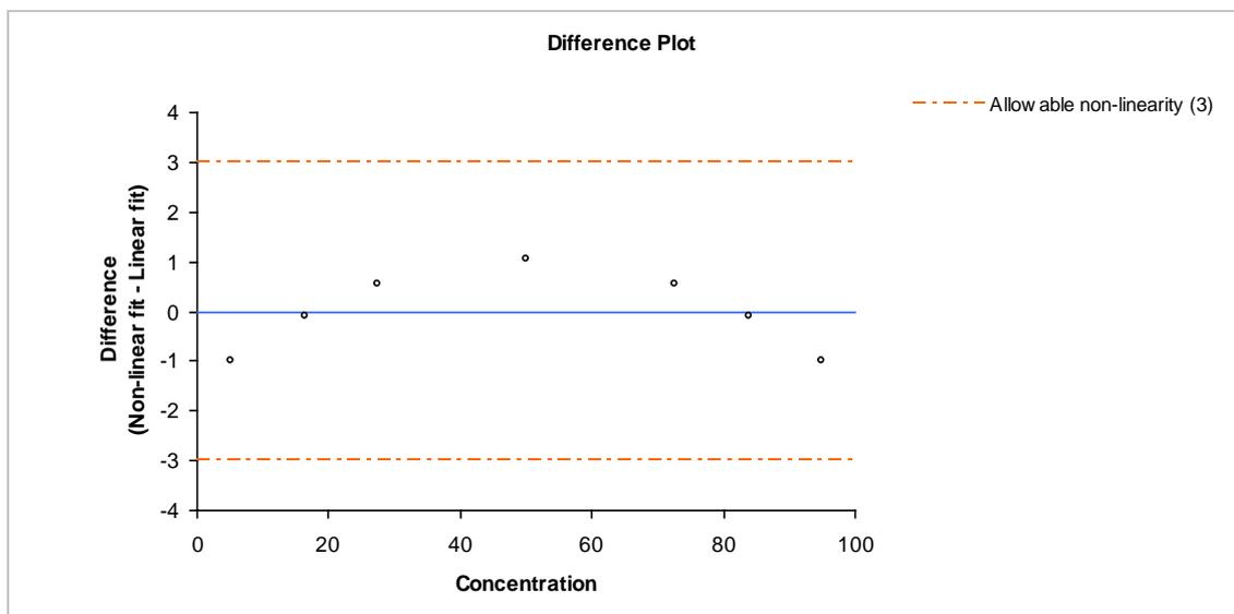
**Figure 6. Example of linearity analysis.** **A** The linear fit and the polynomial fit are shown graphically. The polynomial fit is statistically significant. **B** The difference plot shows that the data is well within the limits of allowed nonlinearity of 3 percentage units.
