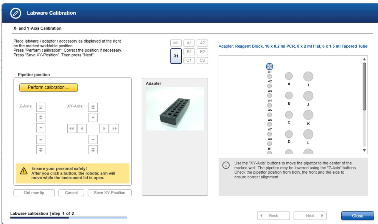
XY-Axis calibration of the reagent block adapter. Position A1 will be used for calibration.
