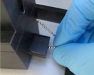
2. Remove the tip ejector by carefully pulling the tip chute upwards.
