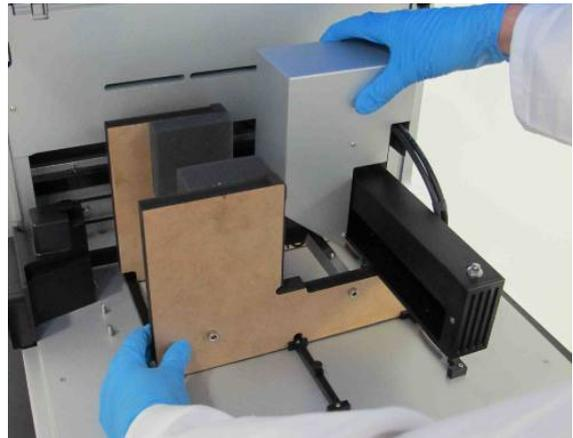
3. Unscrew the Z-axis locking screw. When this screw is removed, the pipettor head will drop.
