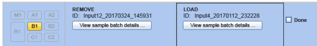
Instruction to load sample batch with ID Input4\_20170112\_232228 to worktable position B1.
