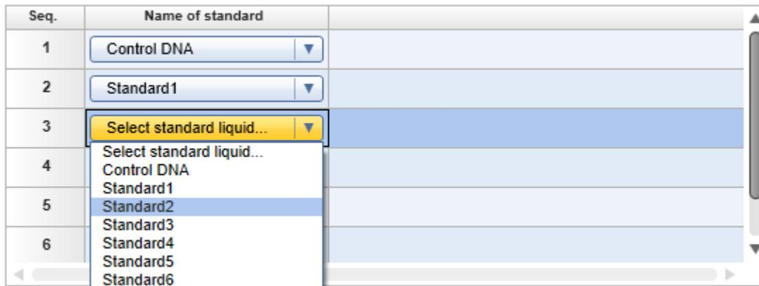
Selecting the appropriate liquid for each standard for a user prepared standard series.
