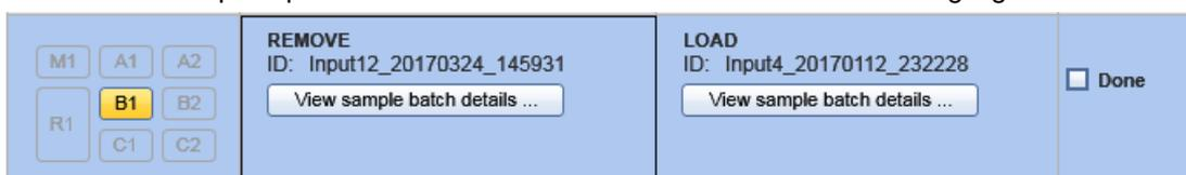
Instruction to remove sample batch with ID Input12\_20170324\_145931 from worktable position B1.
