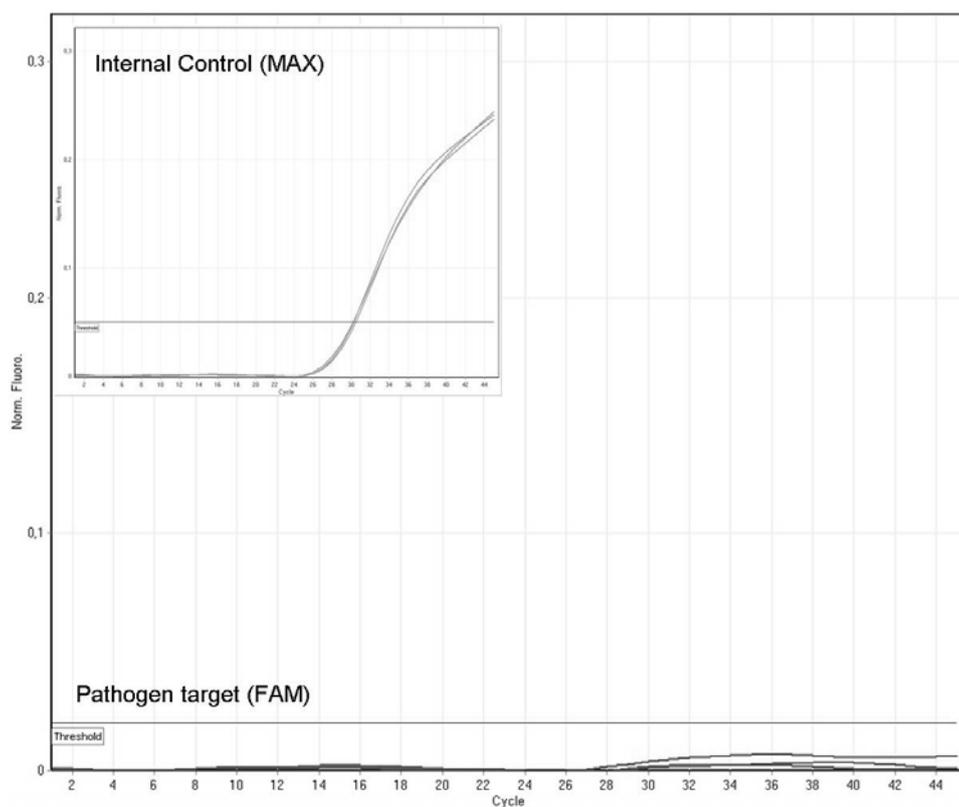
**Figure 5. Typical amplification plots on the Rotor-Gene Q showing no signal for three replicates of a pathogen target with successful amplification of the Internal Control (inset) at the same time, indicating absence of the pathogen target in the sample.**
