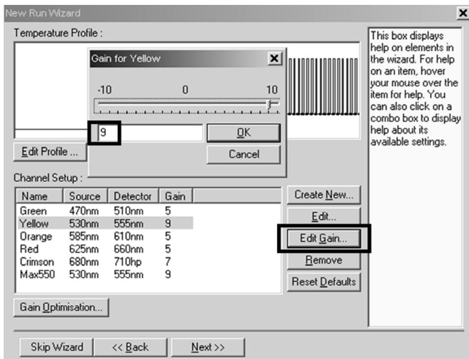
Figure 2. Setting a fixed gain for the Internal Control Assay (yellow channel).
