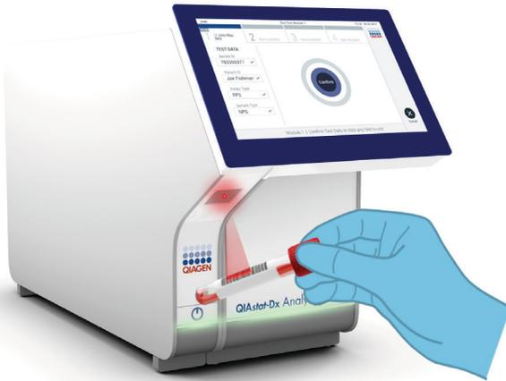
**Figure 11. Scanning sample ID bar code.**
