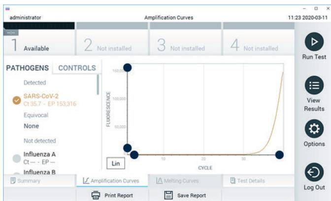
Figure 31. Amplification Curves screen (PATHOGENS tab).
