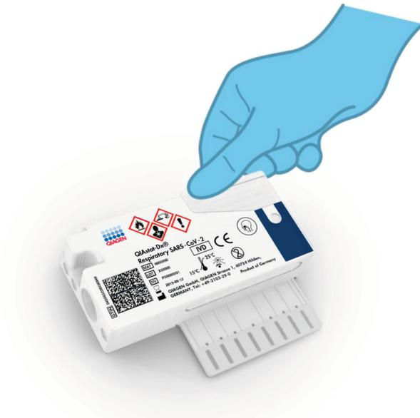
**Figure 22. Closing the sample lid of the main port.**
