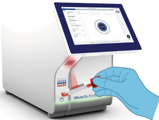
**Figure 24. Scanning sample ID bar code.**
