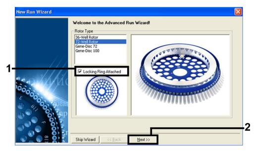
7. First, open the **New Run Wizard** dialog box (Figure 1). Check the **Locking Ring Attached** box and click **Next**.
